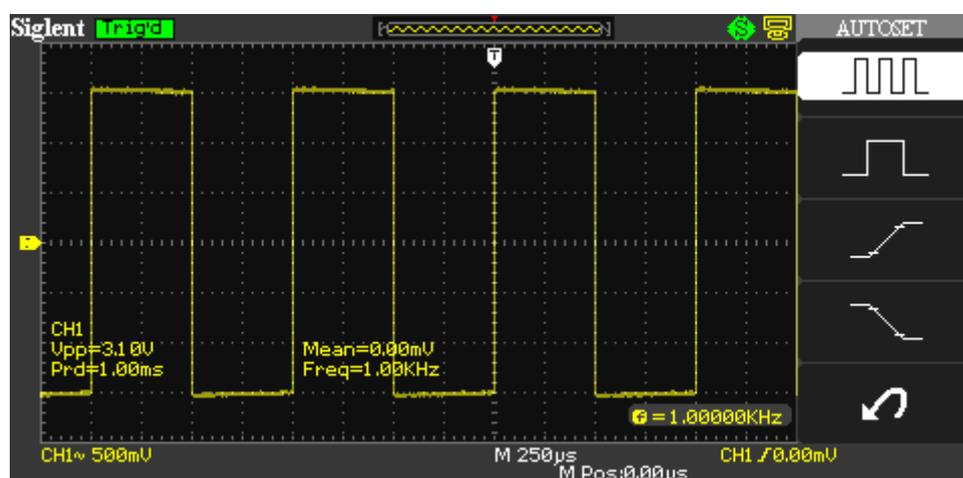
6. Test channel 2 in the same method. If the square waveforms do not display like figure above, please perform “Probe Compensation”.
