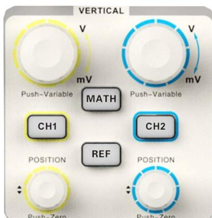
**CH1** **CH2** : Input channels. These two channels are marked with different colors to distinguish different input channels and their waveforms. Pressing the channel button will turn on the corresponding channel as well as its menu, and pressing it twice continuously will turn off the channel.
