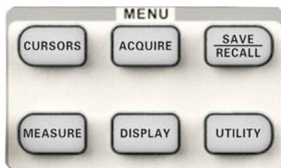
**CURSORS** : Press the button to enter the cursor measurement function menu. The instrument provides three measure modes: Manual, Track and Auto.
