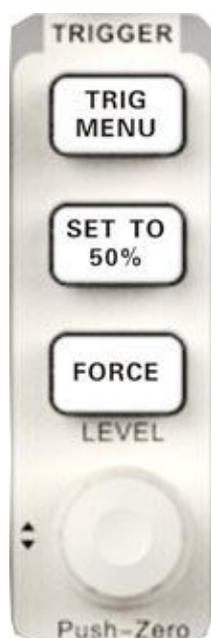
**TRIG MENU** : Press the button to open trigger menu under which five trigger modes are supported.
