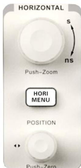
**HORI MENU**: Press the button to open horizontal control menu under which you can turn on/off the delay sweep function and switch the save modes between “long save” and “normal save”.
