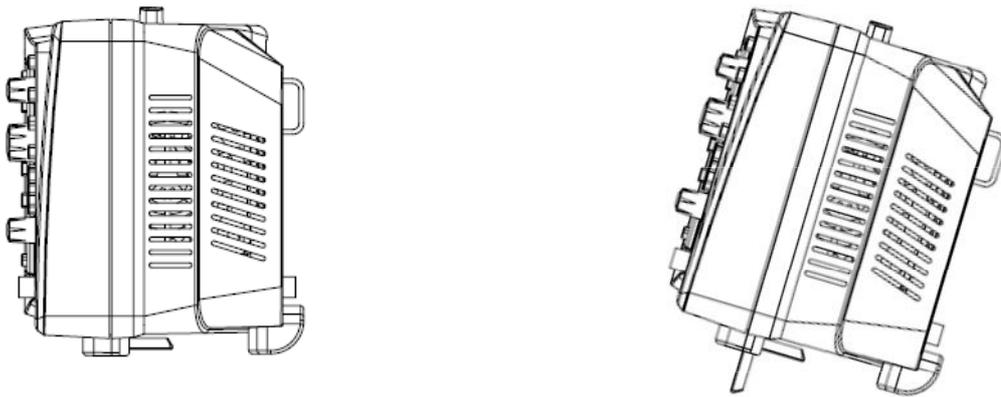
Figure 3 Adjust the Supporting Legs
