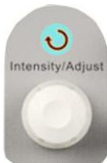
**Adjust waveform brightness** While the light above the knob is dark, adjusting the knob will change the waveform brightness, which ranges from 30%~100%. Turning clockwise means increase while counterclockwise means decrease. You can also select “intensity” in “DISPLAY” menu and then adjust the knob to change the waveform brightness.
